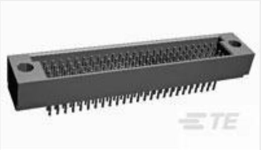
TE Part #532436-2 HDI PIN ASSY 4 ROW 120 POS
