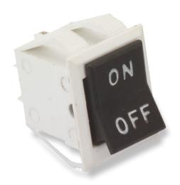
The 610/620-Series switches are double insulated and available in single or double pole configurations. These snap-in mounted switches are offered with either a paddle or rocker actuator and with ratings up to 8 amps.
