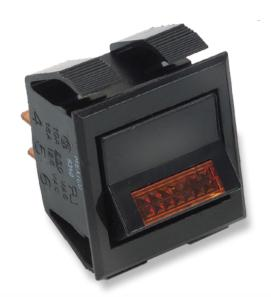
The TG-Series Mid-Sized Tippette rocker switches are single or double pole and feature an all nylon construction. These switches are designed with snap-in mounting for fast, low cost assembly. The illuminated version (LTG) is available with either a paddle or rocker actuator. These AC rated switches are also suitable for low-voltage DC applications assuring compatibility for a wide range of markets.
