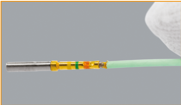
Remove and inspect the completed termination. The contact must have 8 markings, and the wire must be seen in the contact side hole.
