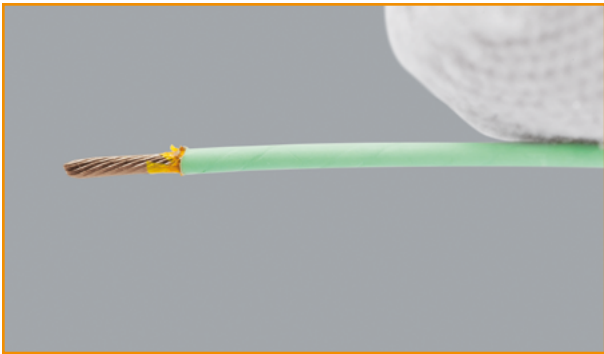
Strip the insulation from the copper wire, with 5 mm maximum strip length. (For aluminum wire, consult TE.)
