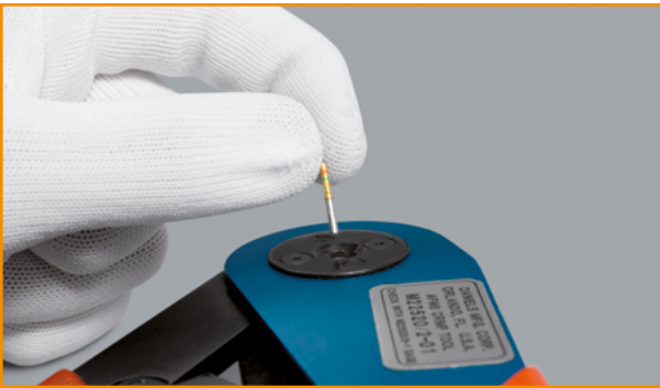
Insert the contact into the crimping tool.
