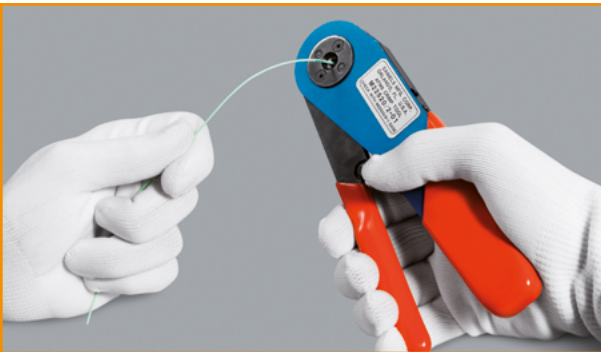
Tighten the crimping tool fully. The handles will not release until the tool is fully bottomed.
