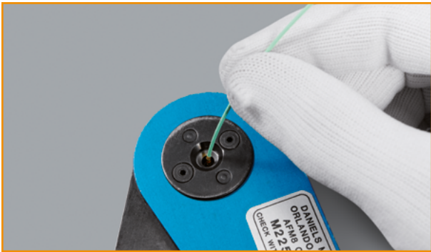
Insert the wire into the contact.
