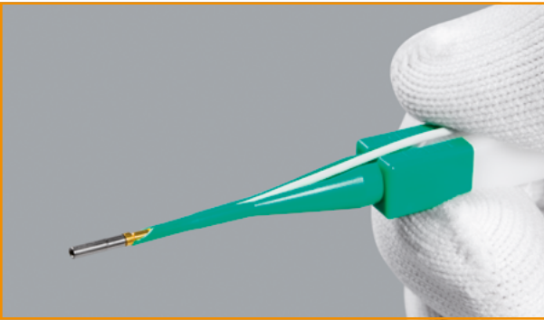
Insert the wire into the slot of the colored end of tool. Pull the wire until the contact butts against the tool.
