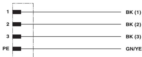
Contact assignment of the M12 connector
