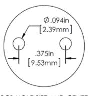
PCB HOLE SIZE AND CENTER TO CENTER SPACING
