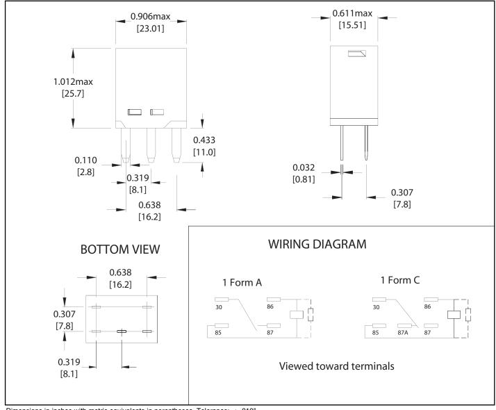
Dimensions in inches with metric equivalents in parentheses. Tolerance:  $\pm$  .010"
