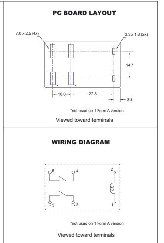
Dimensions in mm. Tolerance:  $\pm$  .25 mm
