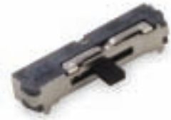
JSM07011SAQN SP3T Surface Mount Momentary one side & Maintained the other
