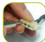
Put the pin extractor into housing
