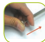
Push the plunger of pin extractor
