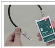
BNC cable test
