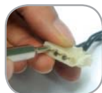
Put the pin extractor into housing
