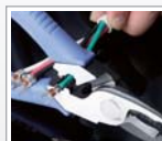
Crimping non-insulated terminals
