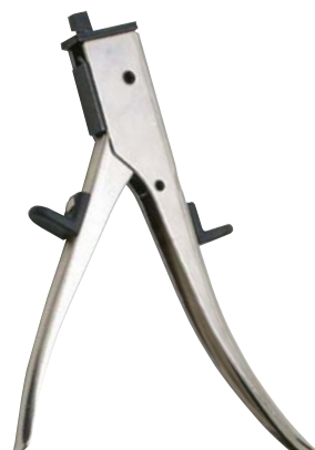
A scribe line can be followed by locking down on work in this position. A slot is cut by making successive cuts.
