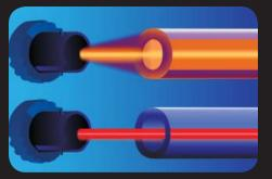
LED spot size:  $>100\mu m$ , 62.5/125 fiber. Laser spot size:  $\sim30\mu m$ , 50/125 fiber.
