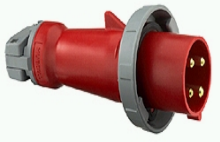
Watertight IEC Pin and Sleeve Plug, 4P5W, 100A 3PH 347/600V
