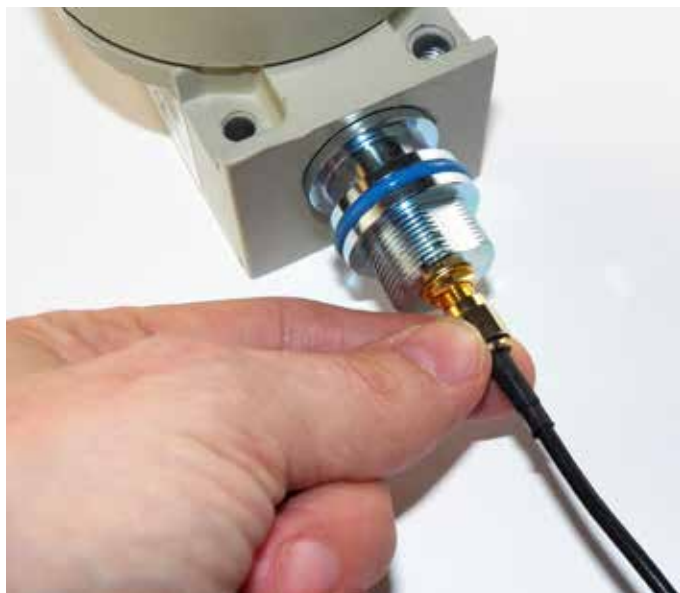
Figure 8. ISA100 Wireless WBX RP-SMA Connection, Remote
