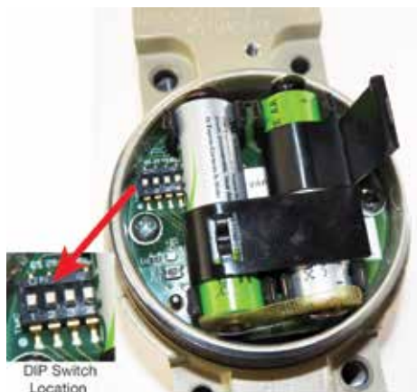
Figure 11. DIP Switch Settings
