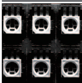
Positioning of LED Packages
