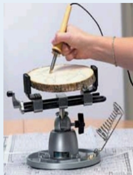
The Model 350 Multi-Position Work Center holds large objects and comes with the large diameter 312 Base Tray Mount for added stability.
