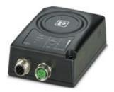
Combined Ethernet wireless module with Bluetooth and Wi-Fi, internal antenna, Wi-Fi: AP and client, 2.4 and 5 GHz, Bluetooth: 2.1+EDR/4.0, PAN up to 7 connections, IP65, 9 ... 30 V DC, M12 connection, WEB, AT commands and mode button
