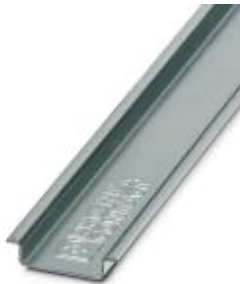
DIN rail, unperforated, Standard profile, width: 35 mm, height: 7.5 mm, acc. to EN 60715, material: Steel, Galvanized, white passivated, length: 2000 mm, color: silver
