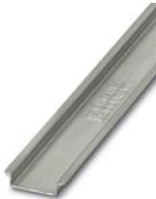
DIN rail, material: steel, unperforated, height: 7.5 mm, width: 35 mm, length: 1 m
