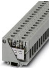
Mini feed-through terminal block, Connection method: Screw connection, Cross section: 0.5 mm 2 - 10 mm 2 , AWG: 20 - 8, Width: 7.5 mm, Color: gray, Mounting type: NS 15
