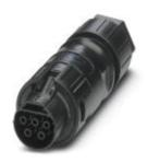
Circular connectors (cable-side), Range of articles: PRC, Coupler connector, type: Can only be released with a tool, housing material: PPE, color: black, number of positions: 5, min. conductor cross section: 1.5 mm², max. conductor cross section: 6 mm², nom. voltage: 690 V AC, rated current: 35 A, Connection method: Screw connection, Type of contact: Socket, min. cable diameter: 12 mm, max. cable diameter: 16 mm
