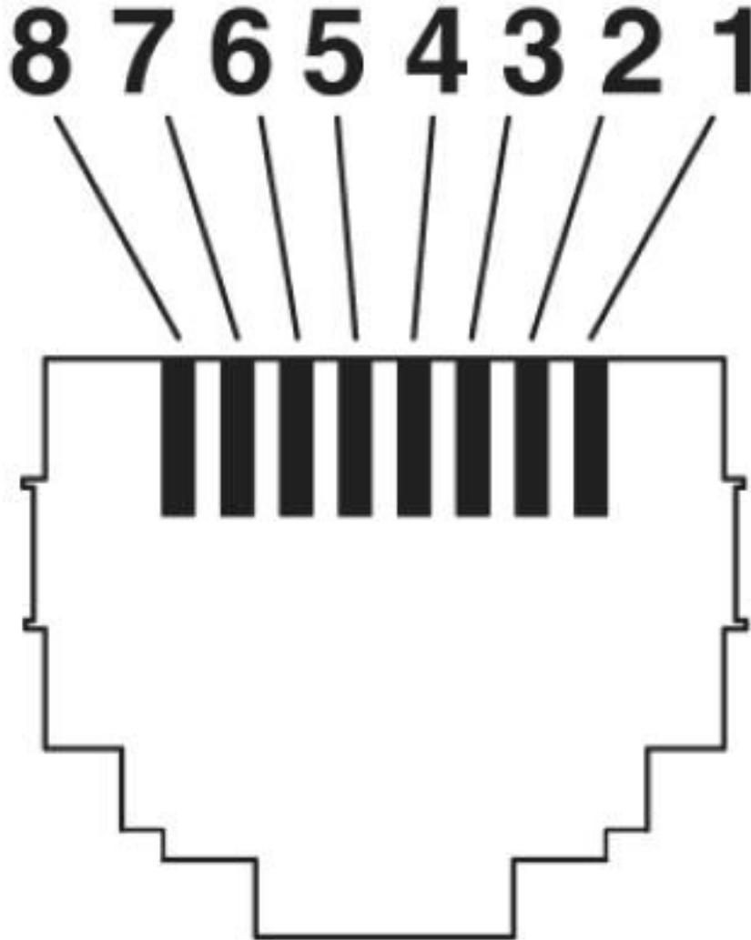
Connector pin assignment plug RJ45
