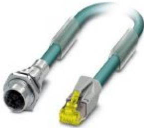
Assembled Ethernet cable, CAT6<sub>A</sub>, shielded, 4-pair, M12 flush-type socket, rear/screw mounting with M16 thread to RJ45/IP20 connector, length: 1 m
