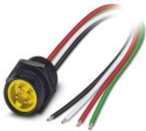
Sensor/actuator flush-type plug, 4-pos., 7/8", front mounting with 7/8" fastening thread, with 1.0 m PE litz wire
