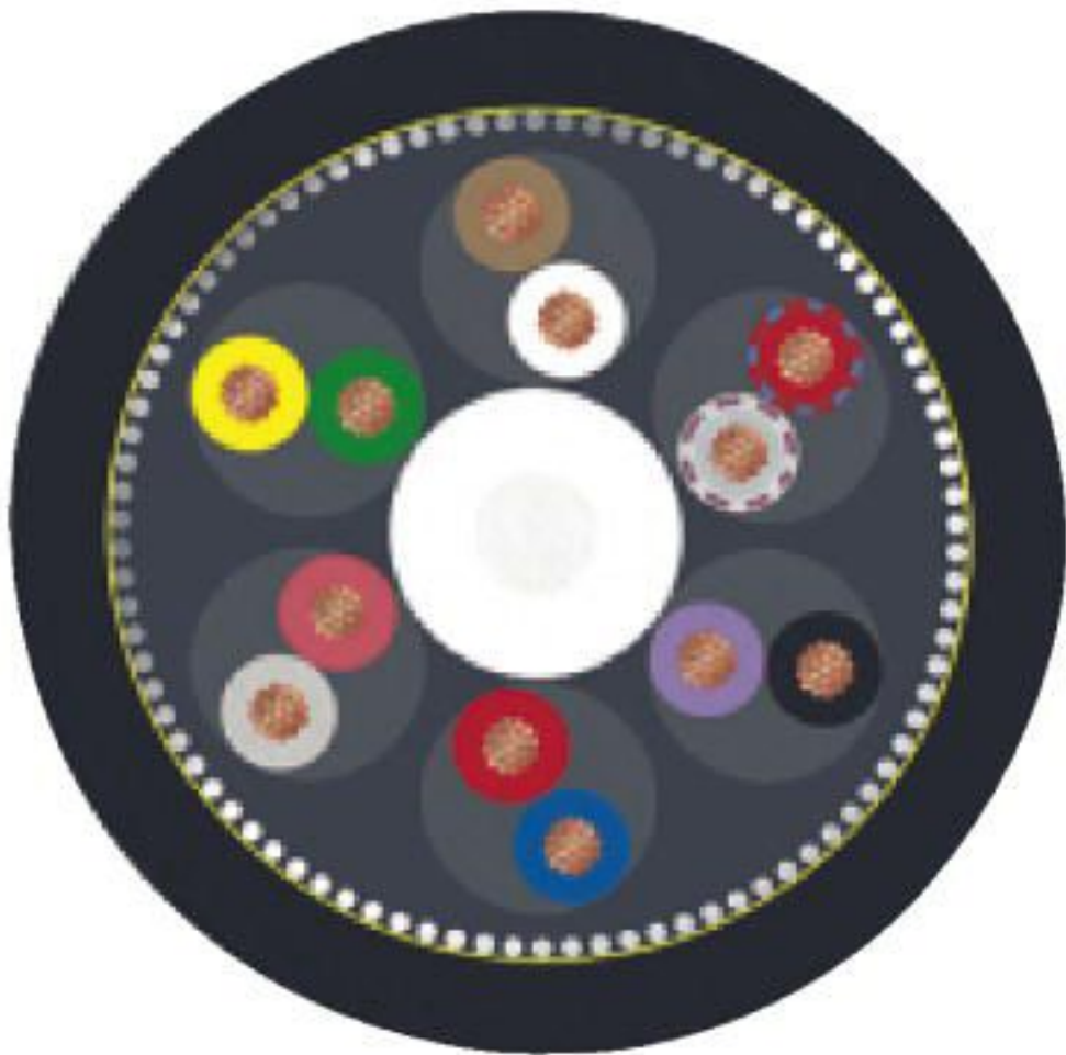
Cable cross section
