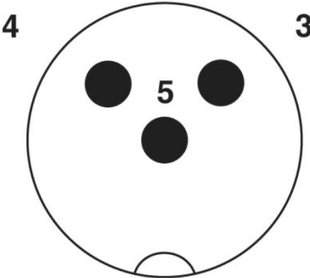
Pin assignment M12 plug, 3-pos., valve connector
