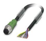
Sensor/actuator cable, 8-position, PUR halogen-free, black-gray RAL 7021, Plug straight M12, A-coded, on free cable end, cable length: 5 m
