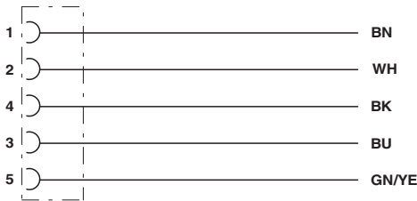
Contact assignment of the M12 socket
