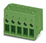
PCB terminal block, nominal current: 32 A, pitch: 7.62 mm, number of positions: 1, connection method: Front screw connection, mounting: Wave soldering, conductor/PCB connection direction: 0°, color: green. The article can be aligned to create different nos. of positions!
