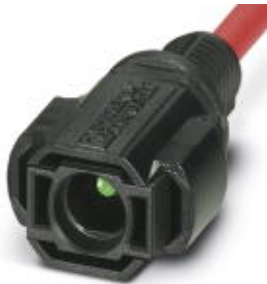
Photovoltaic connector, Nominal current: 27 A, Nom. voltage: 1500 V, Connection type: Crimp, Color: black, Can only be released using a tool
