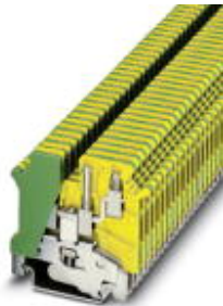
1-level ground modular terminal block with single-sided double connection, cross section: 0.2 - 2.5 mm 2 , width: 5.2 mm, color: green-yellow
