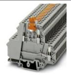
Feed-through terminal block, With test socket screws for insertion of test plugs, Connection type: Screw connection, Cross section: 0.2 mm² - 4 mm², AWG: 24 - 12, Nominal current: 26 A, Nominal voltage: 400 V, Length: 80 mm, Width: 6 mm, Color: gray, Assembly: NS 35/7,5, NS 35/15, NS 32
