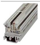
Feed-through terminal block, nominal current: 12 A, nom. voltage: 250 V, cross section: 0.2 mm² - 4 mm² AWG: 24 - 12, mounting type: NS 32, NS 35/15, NS 35/7,5, number of positions: 1, pitch: 5.08 mm, width: 5.08, color: gray
