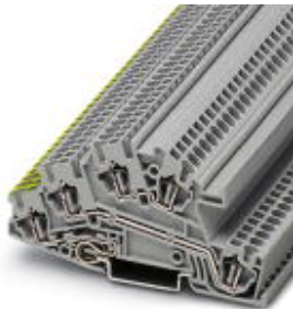
Installation ground terminal block, Spring-cage connection, Cross section: 0.08 mm 2 - 4 mm 2 , AWG: 28 - 12, Width: 5.2 mm, Color: gray, Mounting type: NS 35/7,5, NS 35/15
