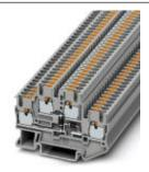
Component terminal block, Connection method: Push-in connection, Cross section: 0.14 mm² - 4 mm², AWG: 26 - 12, Width: 5.2 mm, Color: gray, Mounting type: NS 35/7,5, NS 35/15
