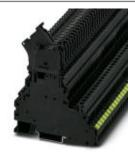
Fuse modular terminal block, fuse type: Glass / ceramics / ..., connection method: Screw connection, cross section:  $0.14 \text{ mm}^2$ -  $6 \text{ mm}^2$ , AWG: 26 - 10, nominal current: 28 A, nom. voltage: 24 V, width: 6.2 mm, fuse type:  $G / 5 \times 20$ , mounting type: NS 35/7.5, NS 35/1.5, color: black
