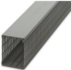
Cable duct, gray, consisting of upper and lower part, width: 80 mm, height: 100 mm, length 2000 mm
