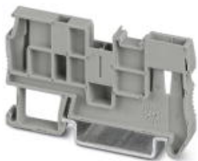
Self-locking flange, Width: 5.2 mm, Height: 35.3 mm, Color: gray, Mounting type: NS 35/7,5, NS 35/15
