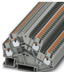
Component terminal block, with integrated diode, Connection method: Push-in connection, Cross section: 0.14 mm 2 - 4 mm 2 , AWG: 26 - 12, Width: 5.2 mm, Color: gray, Mounting type: NS 35/7,5, NS 35/15
