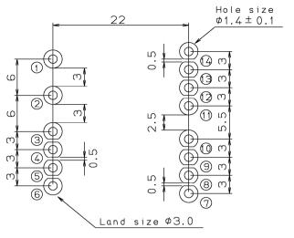
$\ensuremath{\text{\%}}$  The round pulling out figure is a pin numbering.
