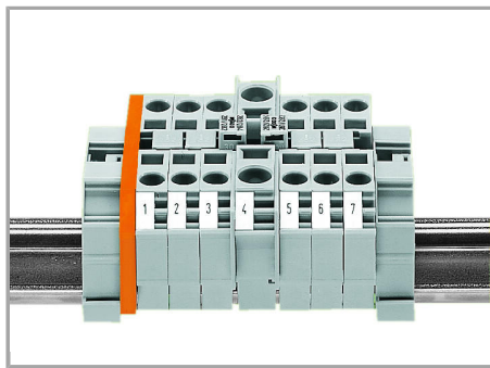
Commoning from 10 mm²/8 AWG (284 Series) to 6 mm²/10 AWG (282 Series) rail-mount terminal blocks via step-down jumpers.
